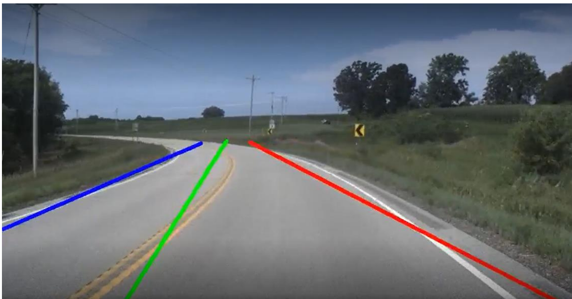
Figure 25 - Example of Tight Curvature Causing Poor Performance
