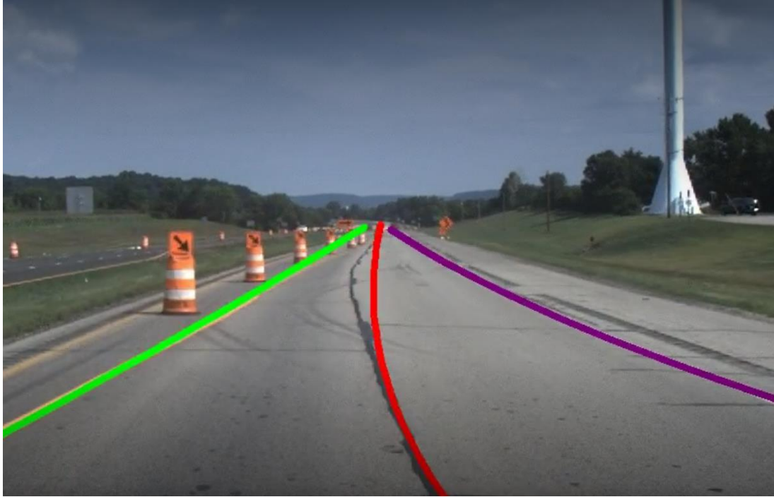
Figure 20 - Misdetection Due to Crack Seal
