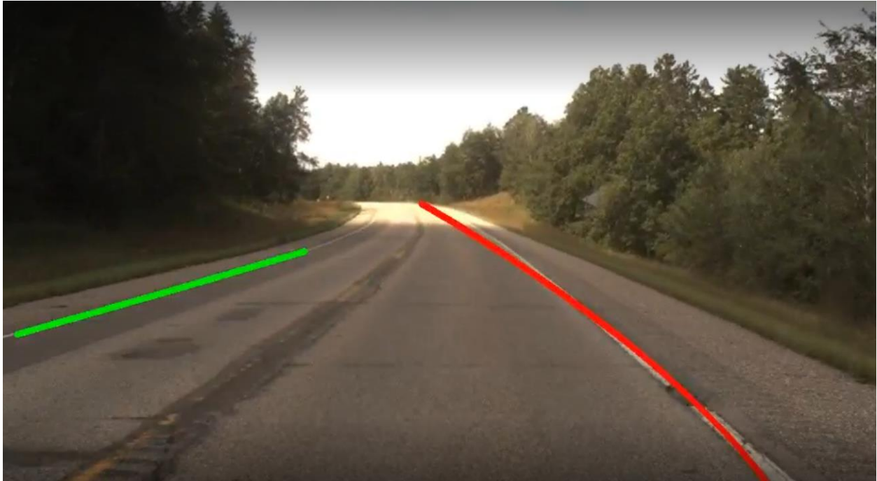
Figure 18 - Example of Poor Lane Line Visibility
