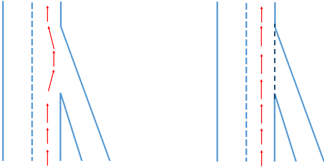
Figure 14 - Entrance Ramp Diagram (Undesirable Vehicle Path on Left, Desired Vehicle Path on Right)
